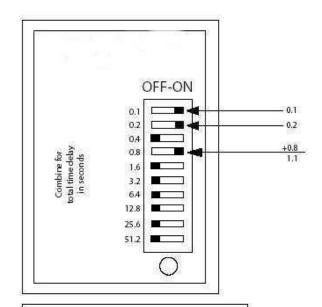
This time delay switch is set to activate a second stage of nitrous after a delay of 1.10 seconds
